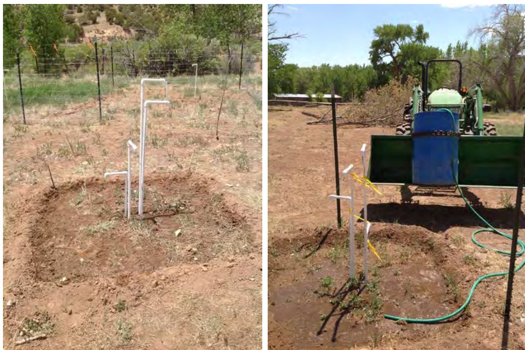
Figure 2-4. Photographs showing the placement of the soil sensors in the control plot (left) and the application of water to the control plot (right).
